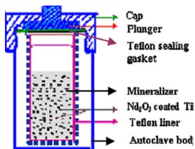
Figure 1 Schematic diagram of hydrothermal autoclave.
